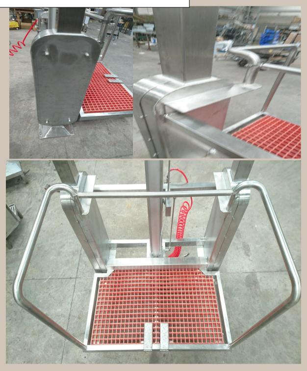
Manlift designed to incorporate Hygiene Facilities incl Sterilizers, Hand Wash Facilities, Apron Washers, Beef Carcass Splitting Saws, SRM Harvesting Manufactured with Bespoke Safety Rails & Safety Harness Facilities. Manlift fitted with anti- vandal concealed Pilot operated foot valves.
