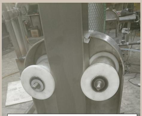
Concealed Inner Carriage with Heavy Duty Machined Rollers with Inner and Outer Stainless-Steel Bearings on 20mm inner Shaft.
